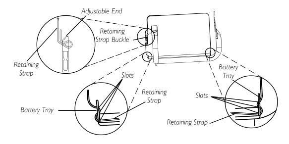
FIGURE 11.10 Replacing Battery Box Retaining Strap
